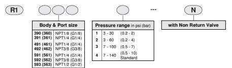
Ordering Example :- Regulator - 3/8 size (with NPT 3/8 (G3/8) port), with pressure range 7 - 100 psi with Non Return Valve Ordering No: R1492 (1462) 3-N.
